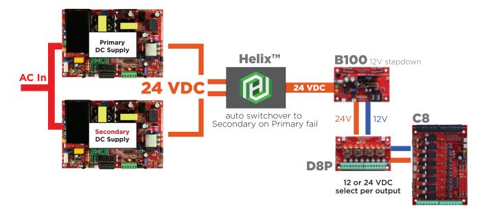
Mercury 8 Door redundant systems provide redundant 24VDC power to the B100, which supplies 12VDC. Both voltages are passed to the D8P and C8 (M8 in managed models).
